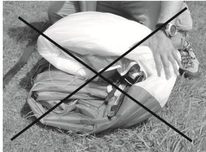
6. Fold the wing up from the trailing edge into 2 or 3 folds, removing excess air and making sure that the packed leading edge is kept flat and outermost. DO NOT fold the leading edge back inside the wing. This may damage / distort the polyamide rods.
